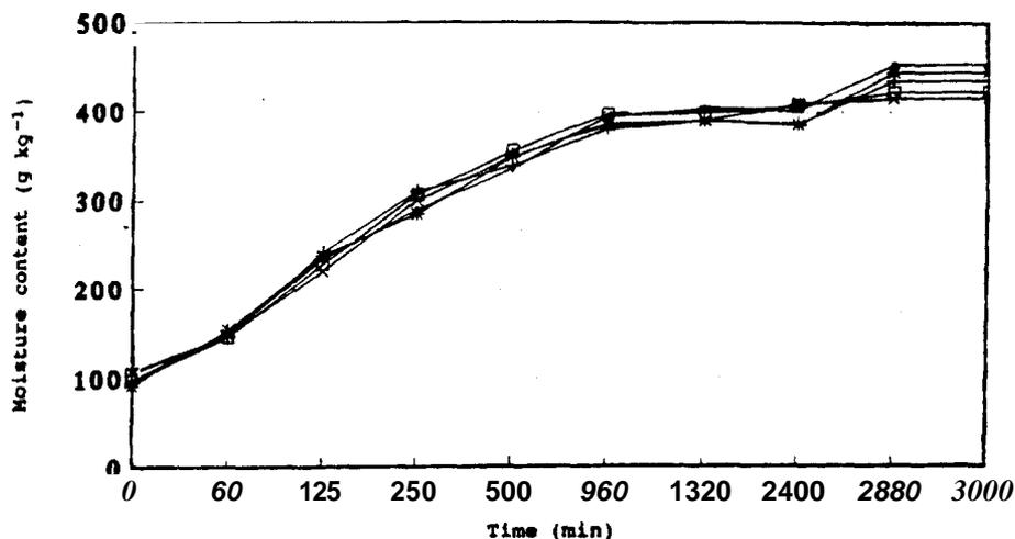
Fig 1. Steeping solution uptake of QPM and normal corns. —□—, QPM White-HO; —+—, QPM Yellow-HO; —\*—, QPM White-C; —○—, H-30; and —x—, H-137.
