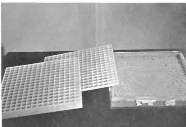
Figure 3. Split cell modules are made from polystyrene light-diffusion louvers.
