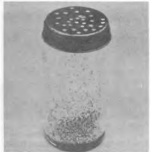
Figure 14. Simple container for efficient infestation with H. zea larvae in rearing containers.
