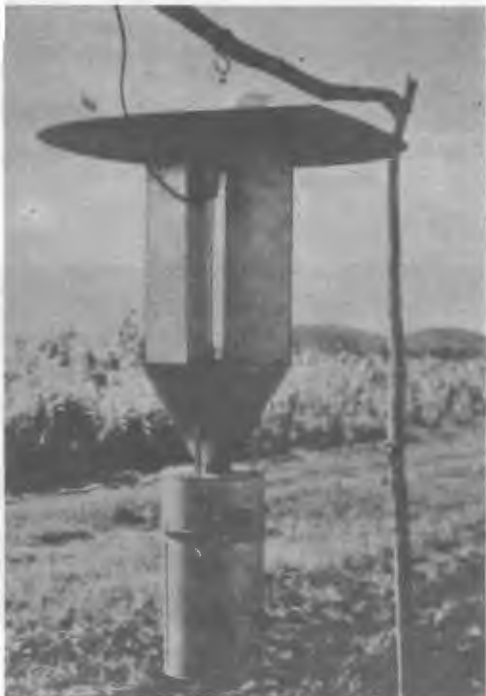
Figure 4. Light trap for collecting H. zea adults for laboratory colony establishment or renovation.
