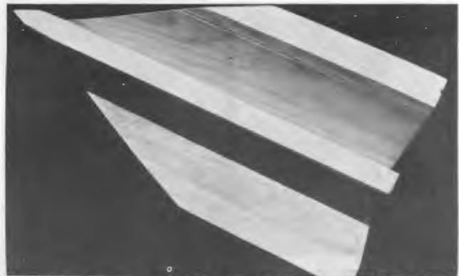
**Photo 3. Upper surface after front V and side pieces sawed.**
