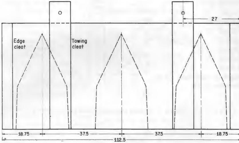
Note: Edge cleats can be eliminated by placing towing cleats at the edge
