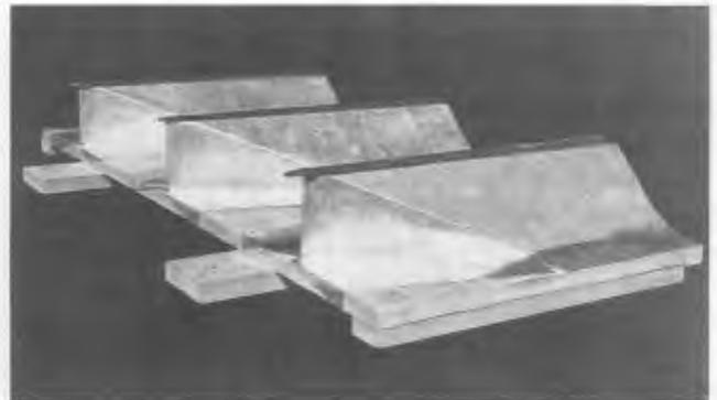
**Photo 6. Note sheet metal overlap at leading edge of V and nailing to front edge of platform.**
