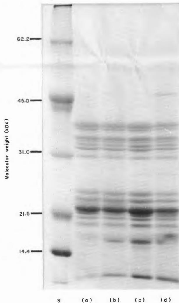
**Fig. 2** Sodium dodecyl sulfate-polyacrylamide gel electrophoresis (SDS-PAGE) patterns of safflower protein isolates. (a) SML-MP; (b) SML-IP; (c) SMI-MP; (d) SMI-IP; (S) Standards. Standard reference proteins: bovine serum albumin, 66.2; ovalbumin, 45; carbonic anhydrase, 31; soybean trypsin inhibitor, 21.5; and lysozyme 14.4 kD (see **Fig. 1** for keys to abbreviations used)
