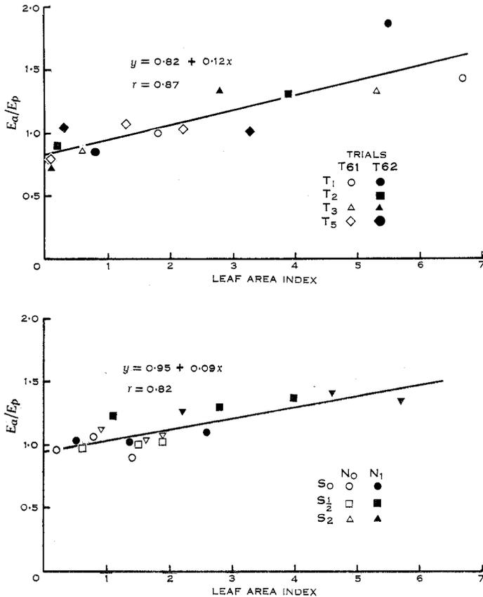
Fig. 5.—Relationship between the ratio of evapotranspiration to pan evaporation ( $E_a/E_p$ ) and leaf area index ( $L$ ) for periods when the crop was adequately supplied with water: trials T61 and T62, and SN62.
