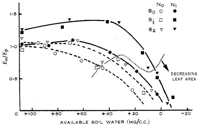
Fig. 6.—Relationship between the ratio of evapotranspiration to pan evaporation ( $E_a/E_p$ ) and available soil water (see text). Unbroken lines represent  $N_1$  treatments and dashed lines  $N_0$  treatments.  $S_1$  and  $S_2$  are considered together, being represented by the same lines. Beneath the dotted line, leaf areas were less than the maximum values for each treatment. Trial SN62.
