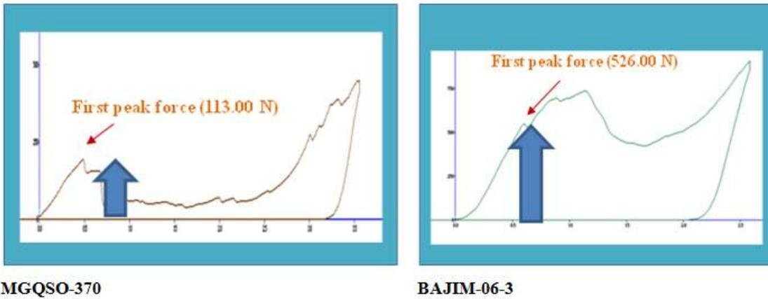
**Figure 4.** Variation for first peak force required to break the grains, an indicator of grain hardness
