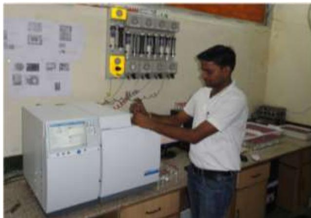
**Figure 1.** Sample feeding in GC for the GHG analysis at DMR laboratory, New Delhi
