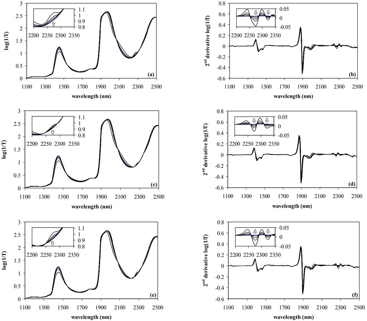
Figure 4. Average spectra of the monocomponent dilution series of some mono- and oligosaccharides; (a) fructose, raw spectra, (b) fructose, second derivative spectra, (c) glucose, raw spectra, (d) glucose, second derivative spectra, (e) sucrose, raw spectra, (f) sucrose, second derivative spectra. The concentration levels of 0, 40, 100, 200 and 400 g L<sup>-1</sup> follow the arrow in enlarged pictures on the top-left corner.
