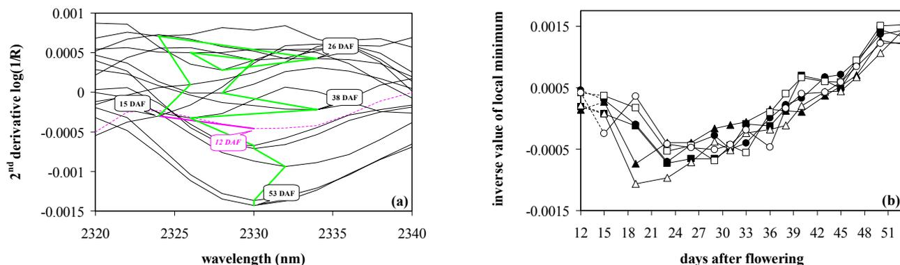
Figure 8. (a) Changes of Carbohydrate III peak in second derivative spectra of wheat seed samples (Jubilejnaja 50) in the 2325–2335 nm region during maturation. broken line=samples of 12 DAF (immature kernels with their bracts). (b) Changes of inverse value of local minimum of Carbohydrate III peak of wheat seed for six varieties during maturation. ■=GK Öthalom, ▲=Bánkúti 1201, ●=Jubilejnaja 50, □=Mv 23, △=Fatima, ○=Mv 15.
