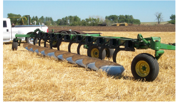
Fig. 3. A large modern moldboard plow used in the north-central U.S. agricultural production areas.
