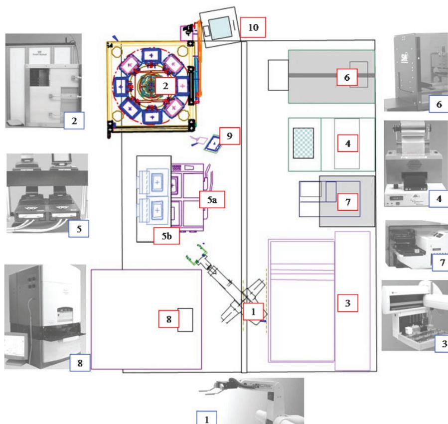
Fig. 2: Illustrated blueprint of the fully automated PCR amplification system
