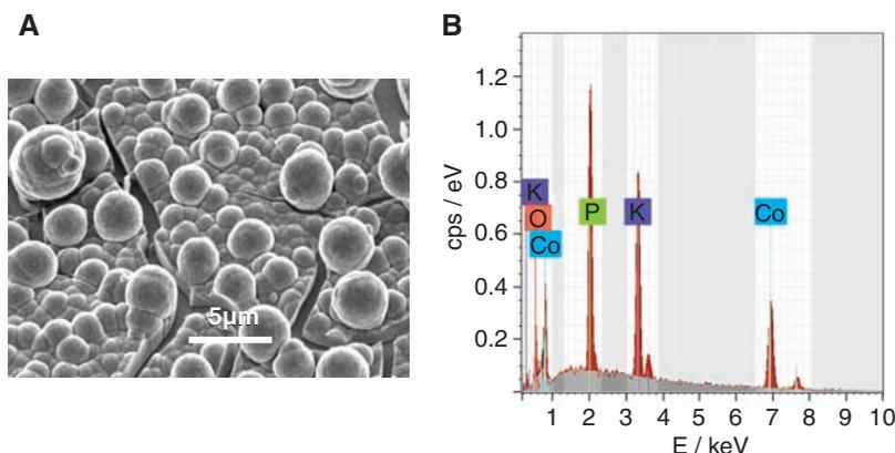
**Fig. 2.** (A) SEM image (30° tilt) of the electrodeposited catalyst after 30 C/cm<sup>2</sup> were passed in 0.1 M KPi electrolyte at pH 7.0, containing 0.5 mM  $\text{Co}^{2+}$ . The ITO substrate can be seen through cracks in the dried film. (B) Typical EDX histogram acquired at 12 kV. cps, counts per second.
