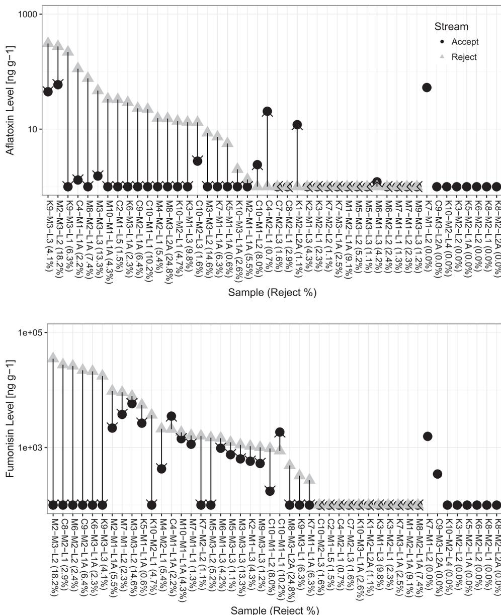
**Fig. 3.** Aflatoxin (top) and fumonisin (bottom) levels in the accept and reject streams of 46 Kenyan market maize samples sorted to removed single kernels with aflatoxin >10 ng g<sup>-1</sup> or fumonisin >1000 ng g<sup>-1</sup>, using the visible to infrared spectrum board (nIRL). A downward pointing arrow indicates that mycotoxin levels were reduced in the accept stream of the sorted maize sample. Points with no detectable mycotoxin are plotted at the LODs.
