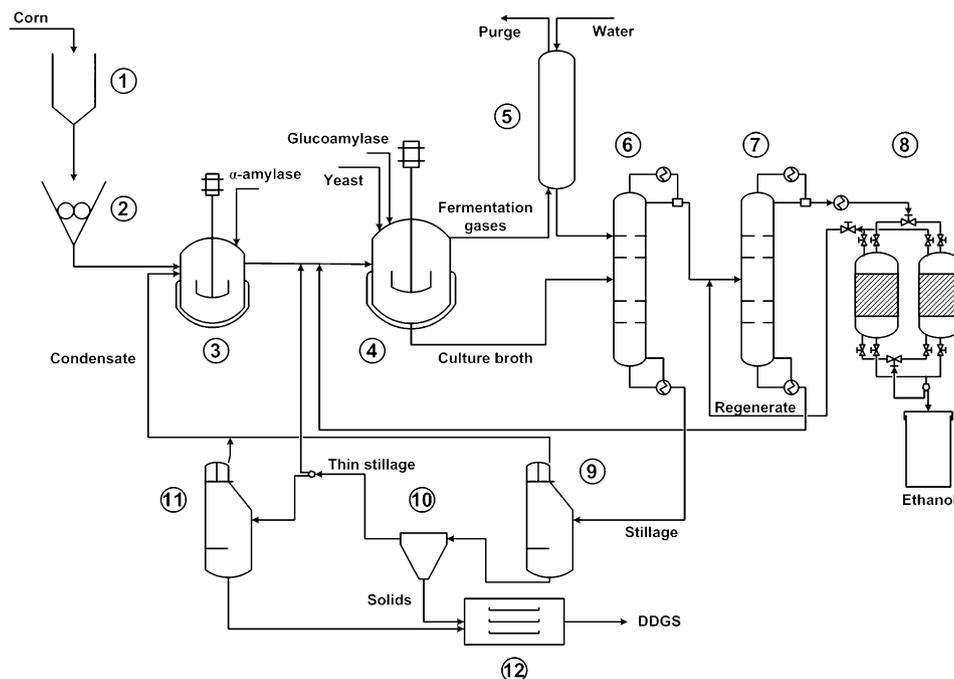
Fig. 1. Simplified flowsheet of fuel ethanol production from corn. 1. Washing tank, 2. Crusher, 3. Liquefaction reactor, 4. SSF reactor, 5. Ethanol absorber, 6. Concentration column, 7. Rectification column, 8. Molecular sieves, 9. First evaporator train, 10. Centrifuge, 11. Second evaporator train, 12. Dryer.
