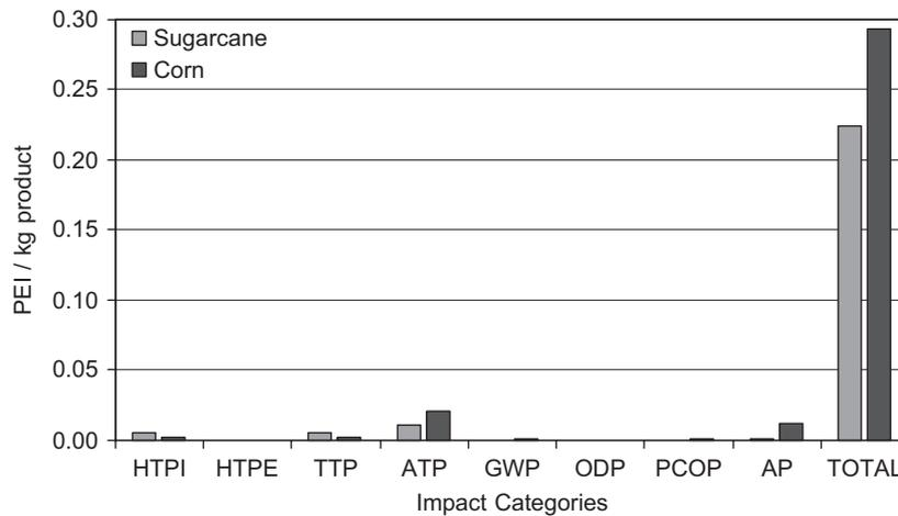
Fig. 5. Total output rate of environmental impact for the studied processes. The impact is expressed as the PEI leaving the system per mass of product streams.
