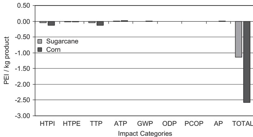
Fig. 6. Potential environmental impact generated within the studied processes. The impact is expressed as the PEI generated within the process per mass of product streams.
