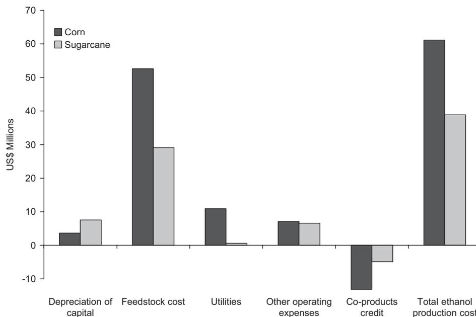
Fig. 4. Total production costs of fuel ethanol using corn and sugarcane as raw materials. Operating costs are represented by the feedstock cost, utilities cost and other operating expenses (operating labor, maintenance and operating charges, plant overhead, and general and administrative costs).
