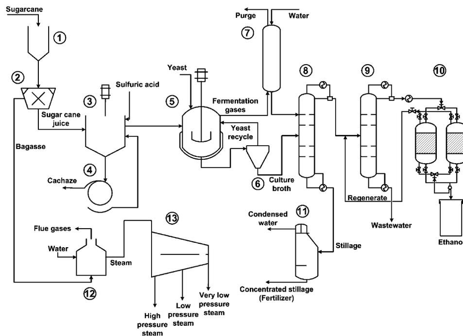
Fig. 2. Simplified flowsheet of fuel ethanol production from sugarcane. 1. Washing tank, 2. Mill, 3. Clarifier, 4. Rotary drum, 5. Fermenter, 6. Centrifuge, 7. Ethanol absorber, 8. Concentration column, 9. Rectification column, 10. Molecular sieves, 11. Evaporator train, 12. Combustor, 13. Turbogenerator.
