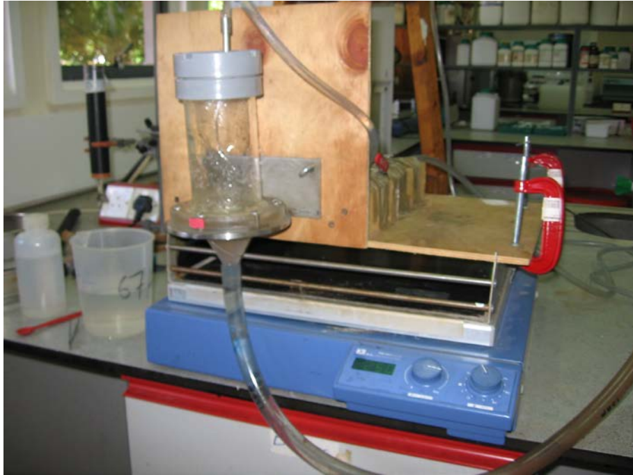
Photo 5: Device used for microaggregate isolation (Isolator) (Six et al., 2000)
